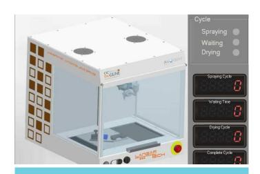
MALDI-TOF. Prototype for Preparation of biological samples.
