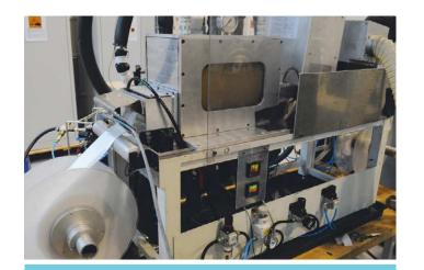
Glass fiber impregnation and curing on-line system
